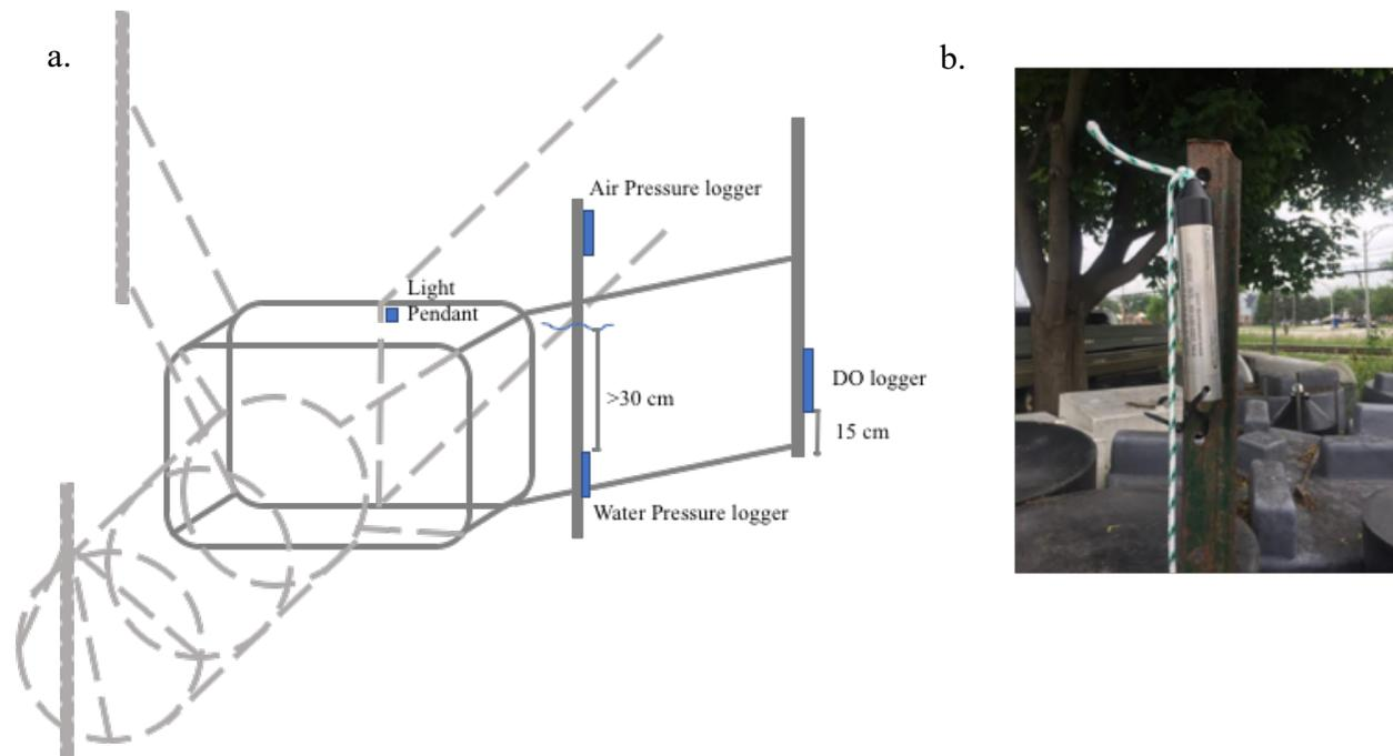
Figure 1a: Diagram of a fyke net with logger locations shown. 1b: An example of a secured logger. A pressure logger secured to a stake with zipties and with bright buoyant cord attached.
